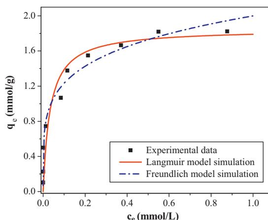
**Fig. 3.** Adsorption isotherm of As(III) on the sorbent. Experimental conditions: sorbent dosage = 0.5 g/L, pH = 8–9, and  $T = 25 \pm 1$  °C.
