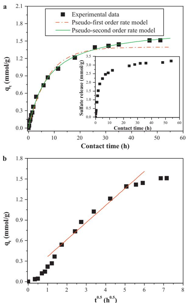
**Fig. 2.** Kinetics study of As(III) adsorption: (a) Experimental data and modeling result by pseudo-first order and pseudo-second order kinetics models (inset graph: release of sulfate); (b) Intraparticle diffusion plot. Experimental conditions: sorbent dosage = 0.2 g/L, initial As(III) concentration = 0.5 mmol-As/L, pH = 8–9,  $T = 25 \pm 1$  °C.
