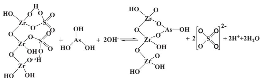
Fig. 7. Schematic diagram of adsorption mechanism of As(III) on the sorbent.
