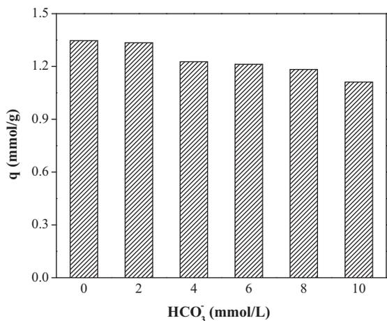
**Fig. 4.** Effect of bicarbonate on the adsorption of As(III). Experimental conditions: initial As(III) concentration = 1.1 mmol/L, solution pH = 8–9, and contact time = 2 days.
