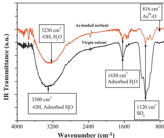
**Fig. 5.** FTIR spectra of virgin and As(III)-loaded sorbent.
