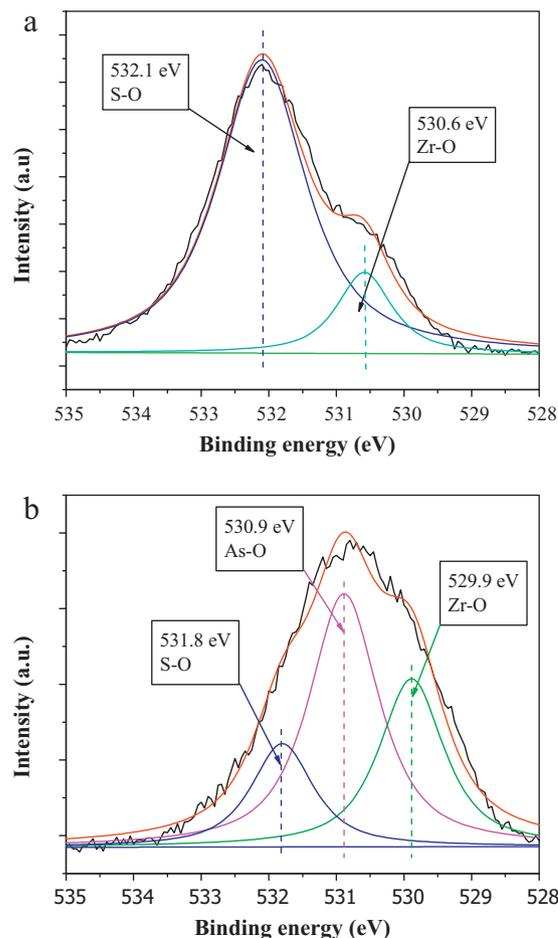
**Fig. 6.** O 1s core-level XPS spectrum of (a) virgin sorbent, (b) As(III)-loaded sorbent.
