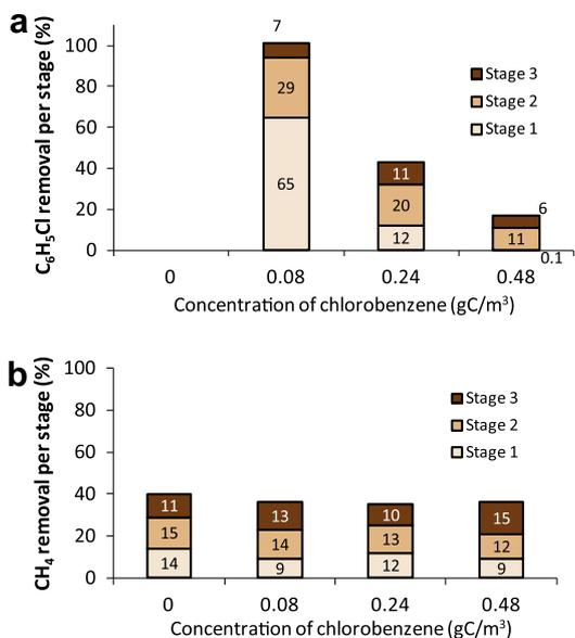
Fig. 6. Chlorobenzene (a) and methane (b) removal per stage as a function of chlorobenzene concentration for BC1.
