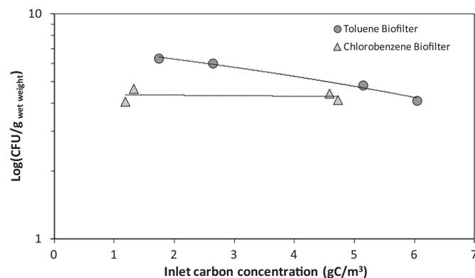
**Fig. 8.** Logarithm of the average Colony Forming Unit of the entire biofilter as a function of the inlet carbon concentration for the toluene-treating biofilter (circle) and the chlorobenzene-treating biofilter (triangle).
