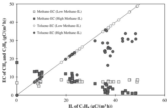
Fig. 2. Elimination capacity of both methane and toluene as a function of inlet load of toluene at methane inlet load of 16  $\text{gC}/(\text{m}^3 \text{ h})$  (low-IL: light color) and 66  $\text{gC}/(\text{m}^3 \text{ h})$  (high-IL: dark color). The dotted line represents the 100% elimination of toluene.
