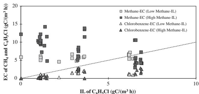
Fig. 3. Elimination capacity of both methane and chlorobenzene as a function of inlet load of chlorobenzene at methane inlet load of 16  $\text{gC}/(\text{m}^3 \text{ h})$  (low-IL: light color) and 66  $\text{gC}/(\text{m}^3 \text{ h})$  (high-IL: dark color). The dotted line represents the 100% elimination of chlorobenzene.
