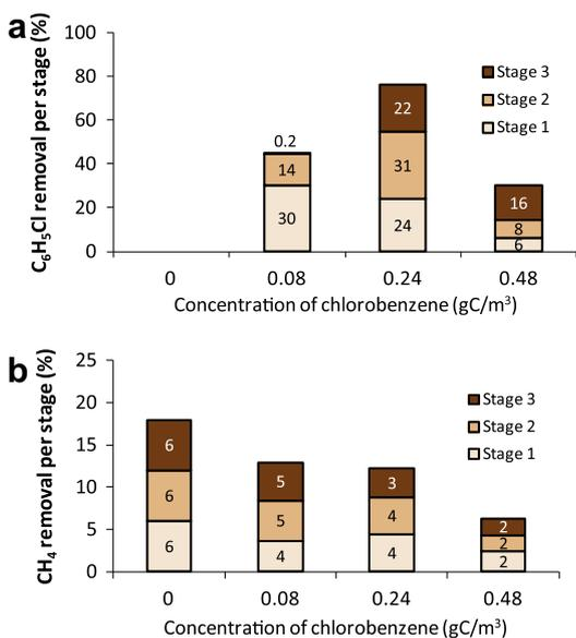
Fig. 7. Chlorobenzene (a) and methane (b) removal per stage as a function of chlorobenzene concentration for BC2.
