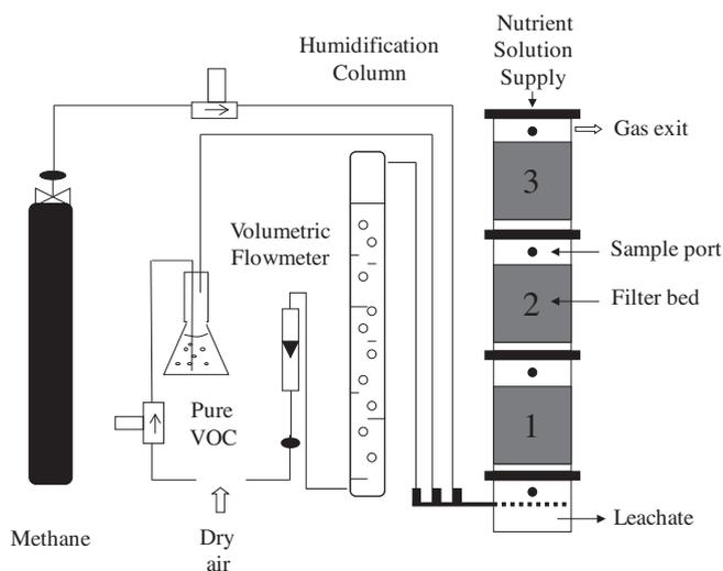
Fig. 1. Experimental set-up of the biofilter. The numbers 1, 2, 3 correspond to the stage number of the biofilter.
