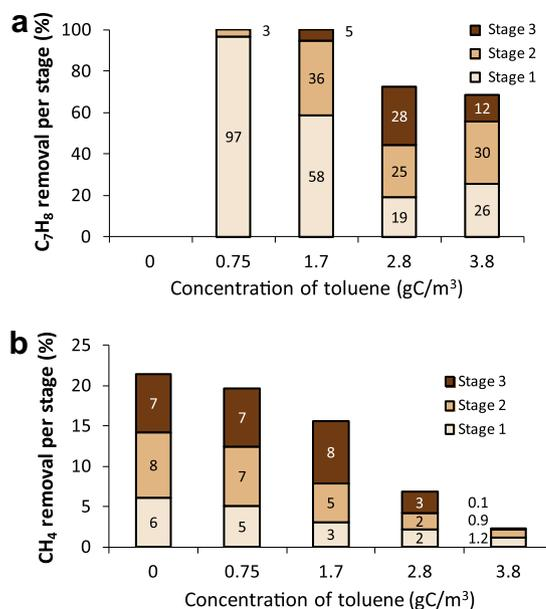
Fig. 5. Toluene (a) and methane (b) removal per stage as a function of toluene concentration for BT2.
