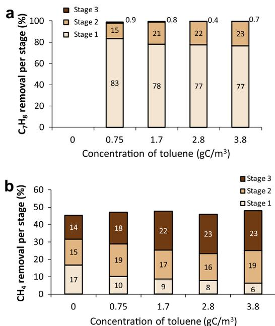
Fig. 4. Toluene (a) and methane (b) removal per stage as a function of toluene concentration for BT1.
