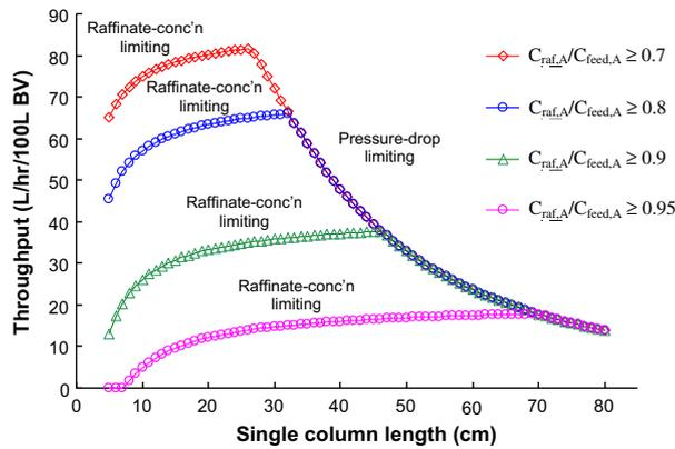
Fig. 4. Effect of the  $C_{raf,A}/C_{feed,A}$  limit on the results from the Case I optimization with the constraint on the raffinate product concentration.
