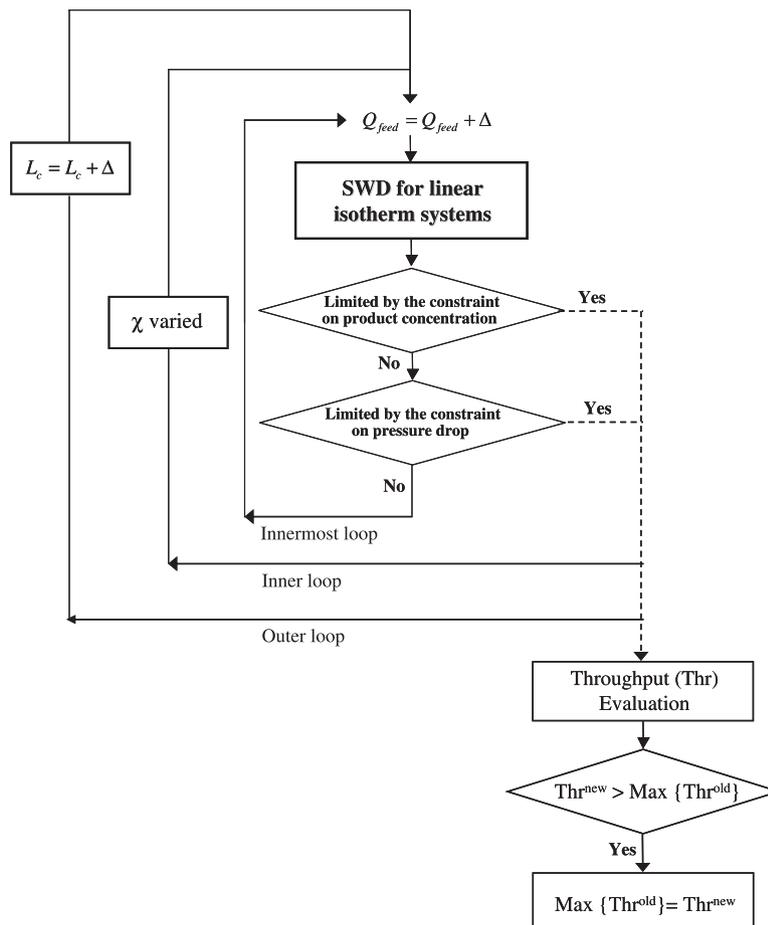
Fig. 2. The overall algorithm of the SWD optimization tool for the SMB process with the requirement on a target level of product concentration.
