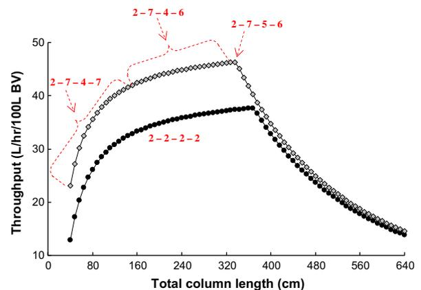
Fig. 6. Comparison of the results from the Case I and II optimizations with the same constraint of  $C_{raf,A}/C_{feed,A} \geq 0.9$ . The black and gray symbols indicate the results from the Case I and Case II optimizations respectively.
