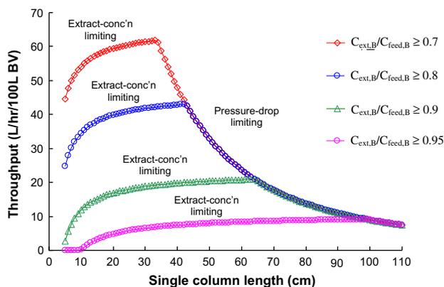
Fig. 5. Effect of the  $C_{ext,B}/C_{feed,B}$  limit on the results from the Case I optimization with the constraint on the extract product concentration.
