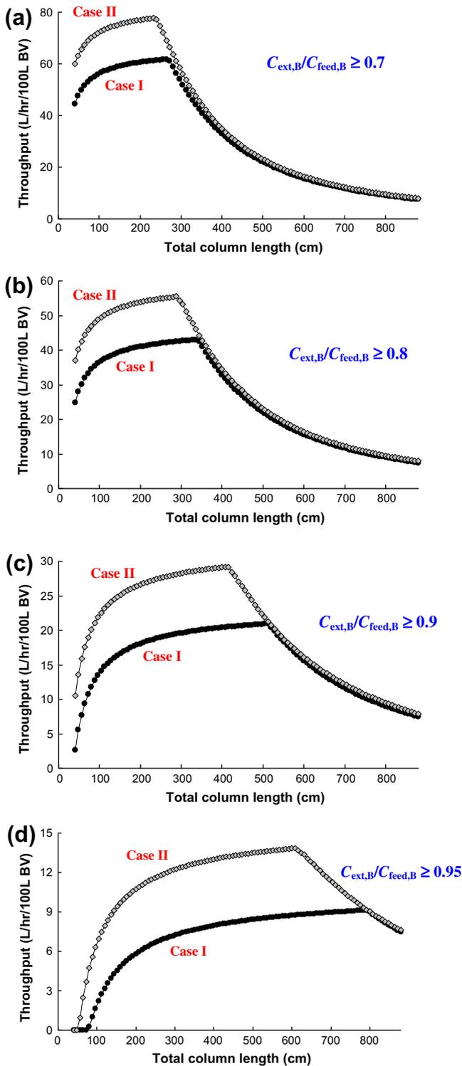
**Fig. 8.** Comparison of the additional results from the Case I and II optimizations with the same constraint of  $C_{ext,B}/C_{feed,B}$ . (a)  $C_{ext,B}/C_{feed,B} \geq 0.7$ , (b)  $C_{ext,B}/C_{feed,B} \geq 0.8$ , (c)  $C_{ext,B}/C_{feed,B} \geq 0.9$ , (d)  $C_{ext,B}/C_{feed,B} \geq 0.95$ . The black and gray symbols indicate the results from the Case I and Case II optimizations respectively.
