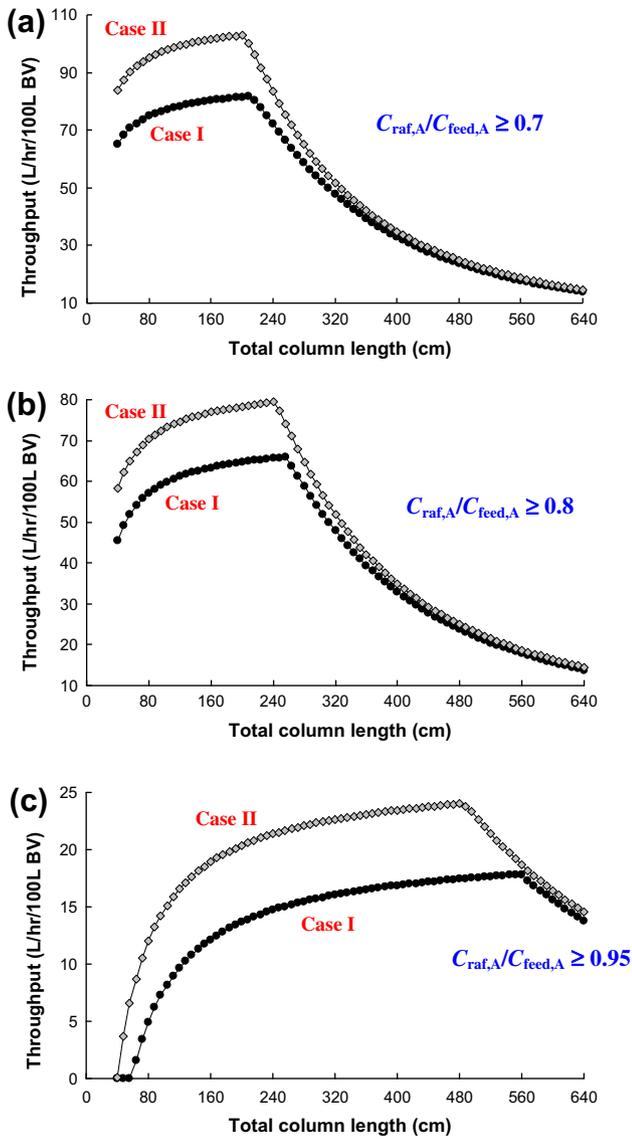
**Fig. 7.** Comparison of the additional results from the Case I and II optimizations with the same constraint of  $C_{raf,A}/C_{feed,A}$ . (a)  $C_{raf,A}/C_{feed,A} \geq 0.7$ , (b)  $C_{raf,A}/C_{feed,A} \geq 0.8$ , (c)  $C_{raf,A}/C_{feed,A} \geq 0.95$ . The black and gray symbols indicate the results from the Case I and Case II optimizations respectively.
