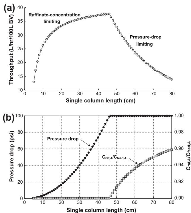
**Fig. 3.** Effect of single column length on the results from the Case I optimization with the constraint of  $C_{\text{raf,A}}/C_{\text{feed,A}} \geq 0.9$ . (a) Throughput, (b)  $C_{\text{raf,A}}/C_{\text{feed,A}}$  and pressure drop.
