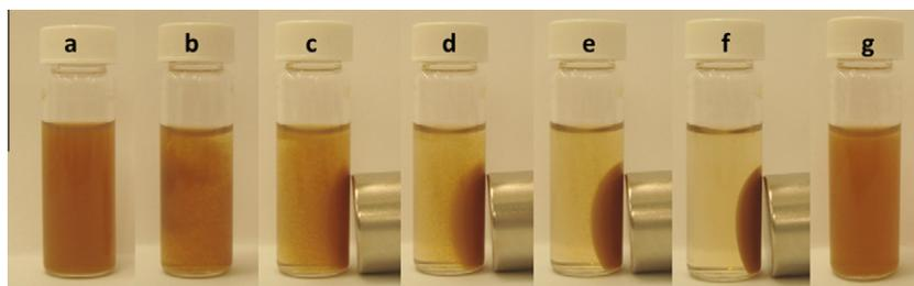
Fig. 4. Photographic images of the behavior of PS@Fe<sub>3</sub>O<sub>4</sub>@GO composite nanoparticles in the magnetic field under different pH conditions: neutral (a), acidic conditions (pH 3–4) (b–f) and a basic condition (pH 8–9) (g). (b–f) correspond to PS@Fe<sub>3</sub>O<sub>4</sub>@GO aqueous suspension after 0 s, 15 s, 30 s, 45 s and 60 s, respectively.
