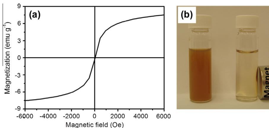
Fig. 3. (a) Magnetization curve of PS@Fe<sub>3</sub>O<sub>4</sub>@GO hybrid, (b) a photograph represents the magnetic separation of PS@Fe<sub>3</sub>O<sub>4</sub>@GO from neutral conditions.
