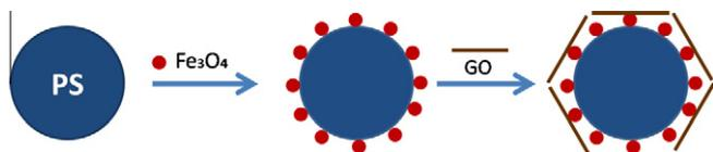
**Scheme 1.** Synthesis procedure of PS@Fe<sub>3</sub>O<sub>4</sub>@GO nanoparticles.
