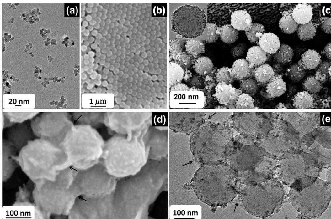
**Fig. 1.** (a) TEM image of Fe<sub>3</sub>O<sub>4</sub> nanoparticles, (b) SEM image of PS nanoparticles, (c) SEM image of PS@Fe<sub>3</sub>O<sub>4</sub>, inset is the corresponding TEM image of PS@Fe<sub>3</sub>O<sub>4</sub>, and (d, e) SEM and TEM images of PS@Fe<sub>3</sub>O<sub>4</sub>@GO, respectively.
