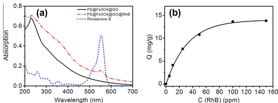
**Fig. 5.** (a) UV-vis spectra of RhB, PS@Fe<sub>3</sub>O<sub>4</sub>@GO and PS@Fe<sub>3</sub>O<sub>4</sub>@GO@RhB. (b) Adsorption isotherms of RhB on PS@Fe<sub>3</sub>O<sub>4</sub>@GO. m/V (for PS@Fe<sub>3</sub>O<sub>4</sub>@GO) = 2 mg/mL, C (RhB) initial = 0–150 ppm, T = 293 K.
