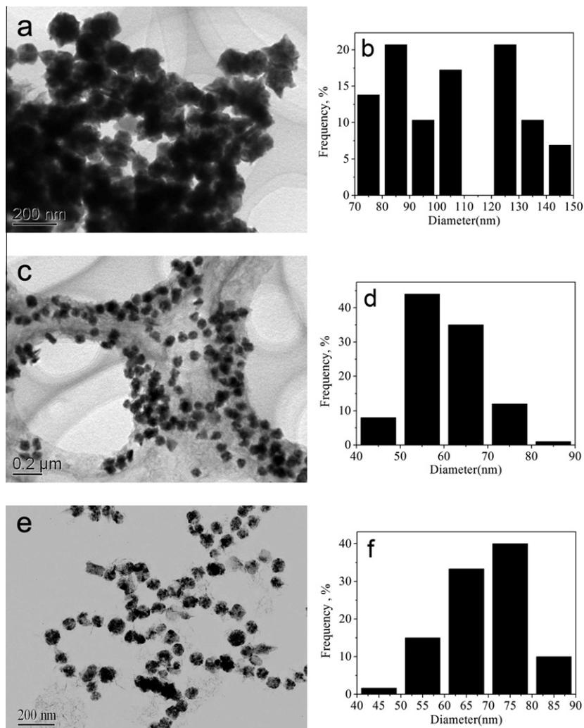
**Fig. 4.** TEM images (a, c, e) and particle size distributions (b, d, f) of nickel nanoparticles prepared using PVP with a PVP/Ni<sup>2+</sup> molar ratio of 0.5 (a, b) and CTAB with a CTAB/Ni<sup>2+</sup> molar ratio of 0.25 (c, d) and a CTAB/Ni<sup>2+</sup> molar ratio of 0.5 (e, f).
