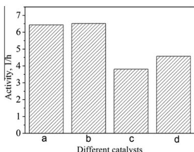
Fig. 6. The catalytic activities of nickel nanoparticles prepared at 70 °C without addition of surfactant (a), with addition of CTAB (b) and PVP (c) and their comparison with that of the commercial used Raney Ni (d).
