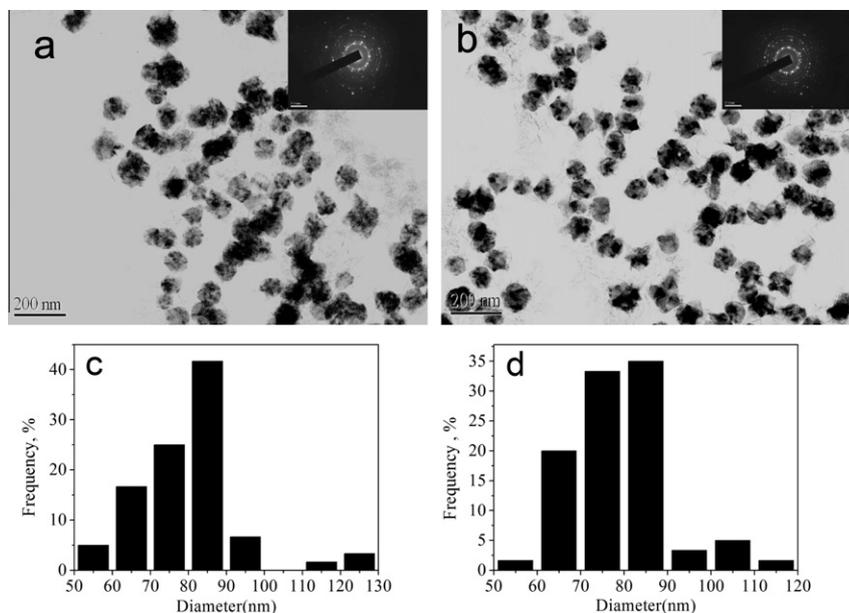
**Fig. 3.** TEM images (a and b) and the corresponding SAED patterns (insets in a and b) and particle size distributions (c and d) of the nickel nanoparticles synthesized at the reaction temperatures of 60 °C (a and c) and 75 °C (b and d).
