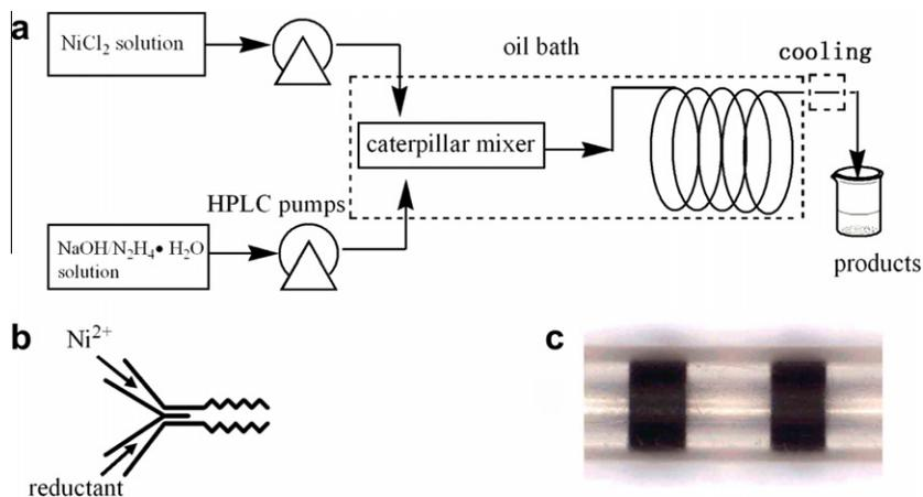
Fig. 1. The schematic of the microreaction process (a), the caterpillar mixer (b), and the flow pattern in the microstructured reactor (c).
