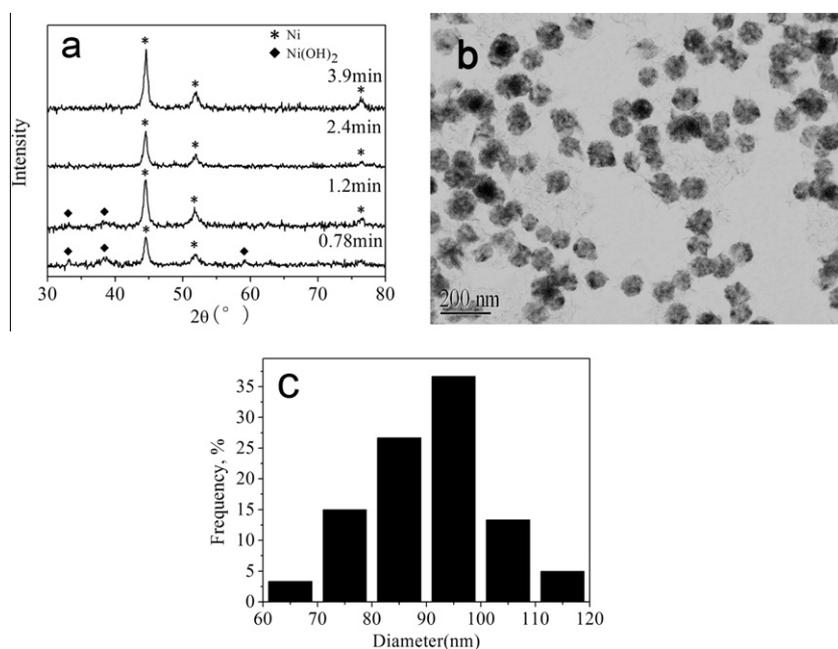
Fig. 2. XRD patterns of the samples produced in the microreactor at 70 °C and different residence times (a) and TEM image (b) and particles size distribution of nickel nanoparticles (c) prepared in the microreactor at 70 °C and a residence time of 3.9 min.
