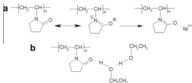
Fig. 5. A proposed mechanism of interaction between PVP and nickel ions (a) and interaction between PVP and ethanol (b).
