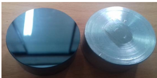
Figure 7. Silicon ingot (left hand side) and aluminum ingot (right hand side)
