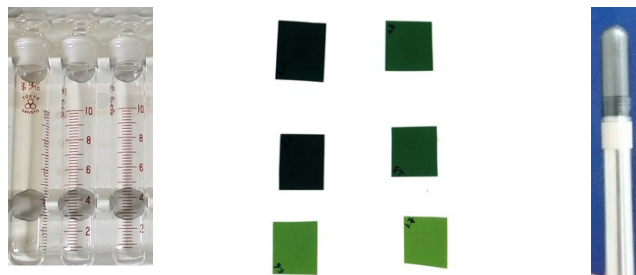
Figure 3: Fricke dosimeter, Gaf chromic film and The TN31013 ion chamber
