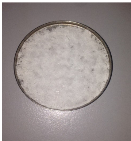
Figure 1. KCl solution was dried up on the planchet
