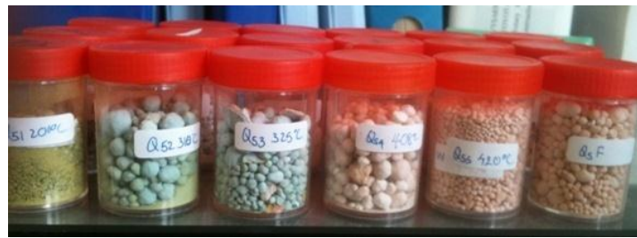
Figure 9. The colours of roasted ore Q5 at different roasting temperatures.
