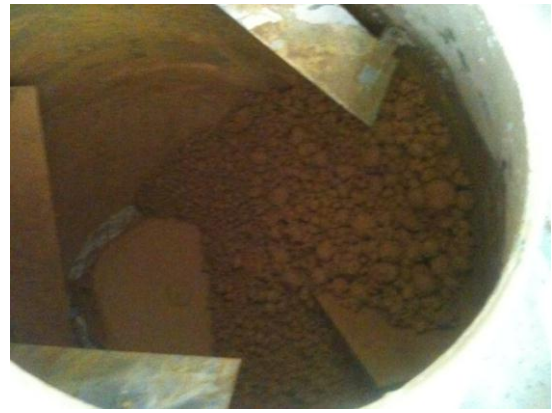
Figure 5. After mixing ore and sulfuric acid with ore/acid rate = 1/1.6 (Q3).
