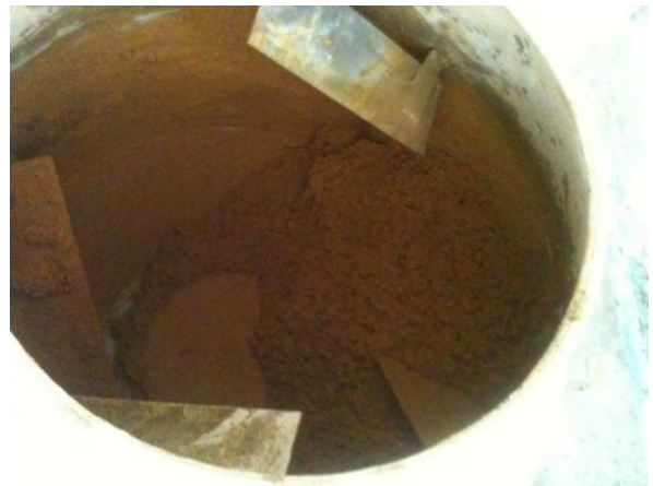
Figure 6. After mixing ore and sulfuric acid with ore/acid rate = 1/1.4 (Q5).
