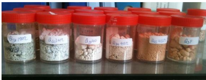
Figure 8. The colours of roasted ore Q3 at different roasting temperatures.
