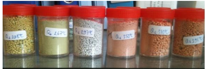
Figure 10. The colors of roasted ore Q6 at different roasting temperatures.
