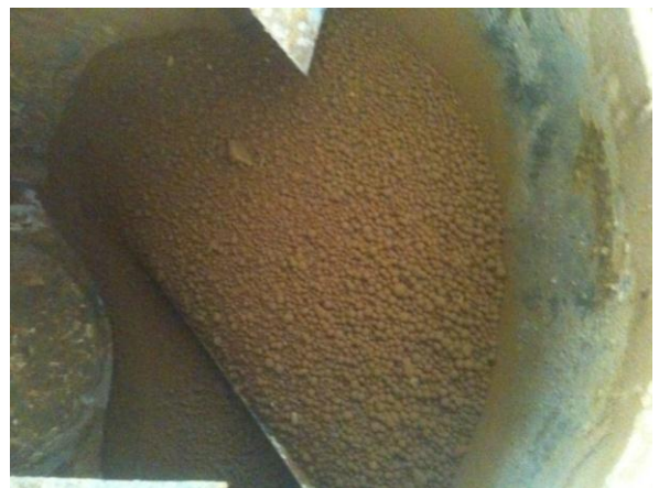
Figure 7. After mixing ore and sulfuric acid with ore/acid rate = 1/1.2 (Q6).
