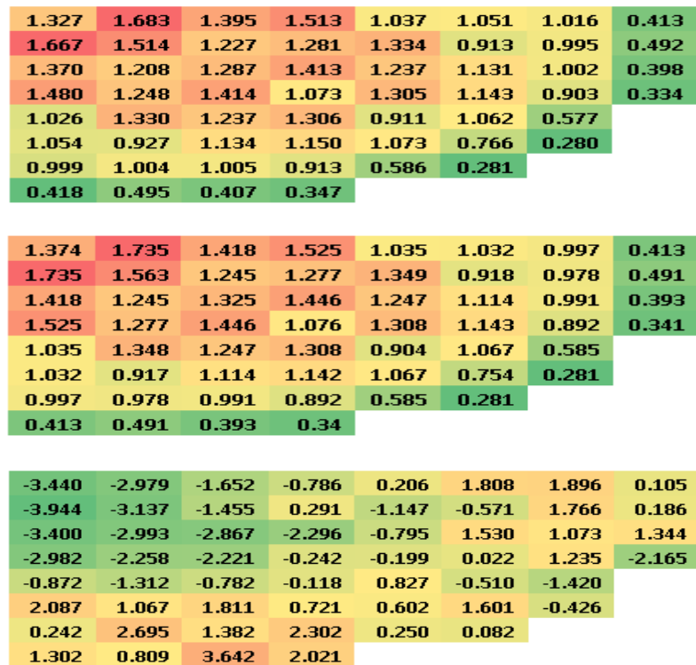
Fig. 3. Assembly power distributions obtained by MCNP6 (this work) (top) and DeCART (middle) and relative difference (%) between MCNP6 and DeCART (bottom) at ARO condition.
