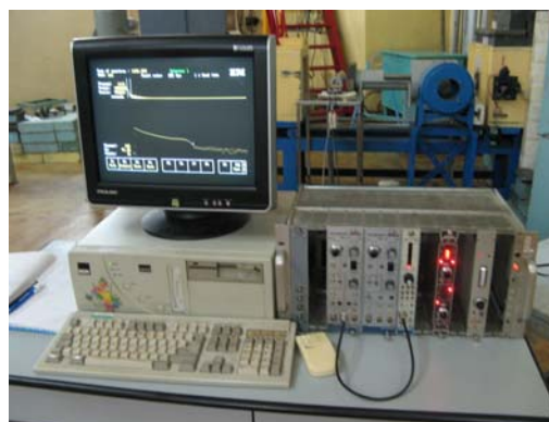
Fig. 3. The new proton recoil spectrometer installed at the Dalat Nuclear research institute.
