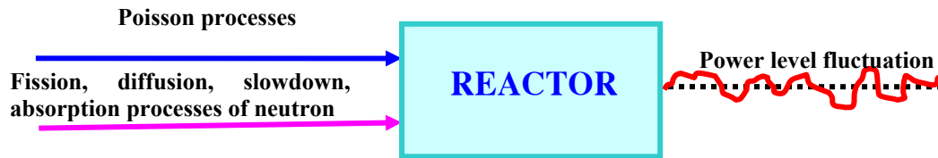
Fig. 1. Model of power level fluctuations in a nuclear reactor
