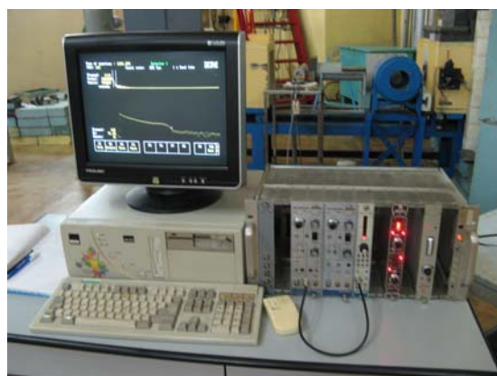
Fig. 3: The new proton recoil spectrometer installed at the Dalat Nuclear Research Institute
