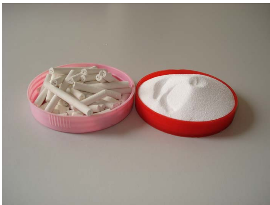
Fig. 2: ZnO catalyst and two holes desulphurization extruder
