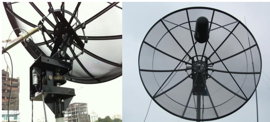
Figure 1. Close-up views of the SRT antenna and of the motor system (gear box and telescopic arm, left panel) and of the feed horn and the calibration antenna (right panel).
