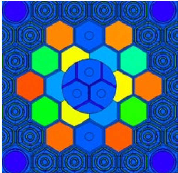
Neutron trap in core configuration of 92 LEU FAs
