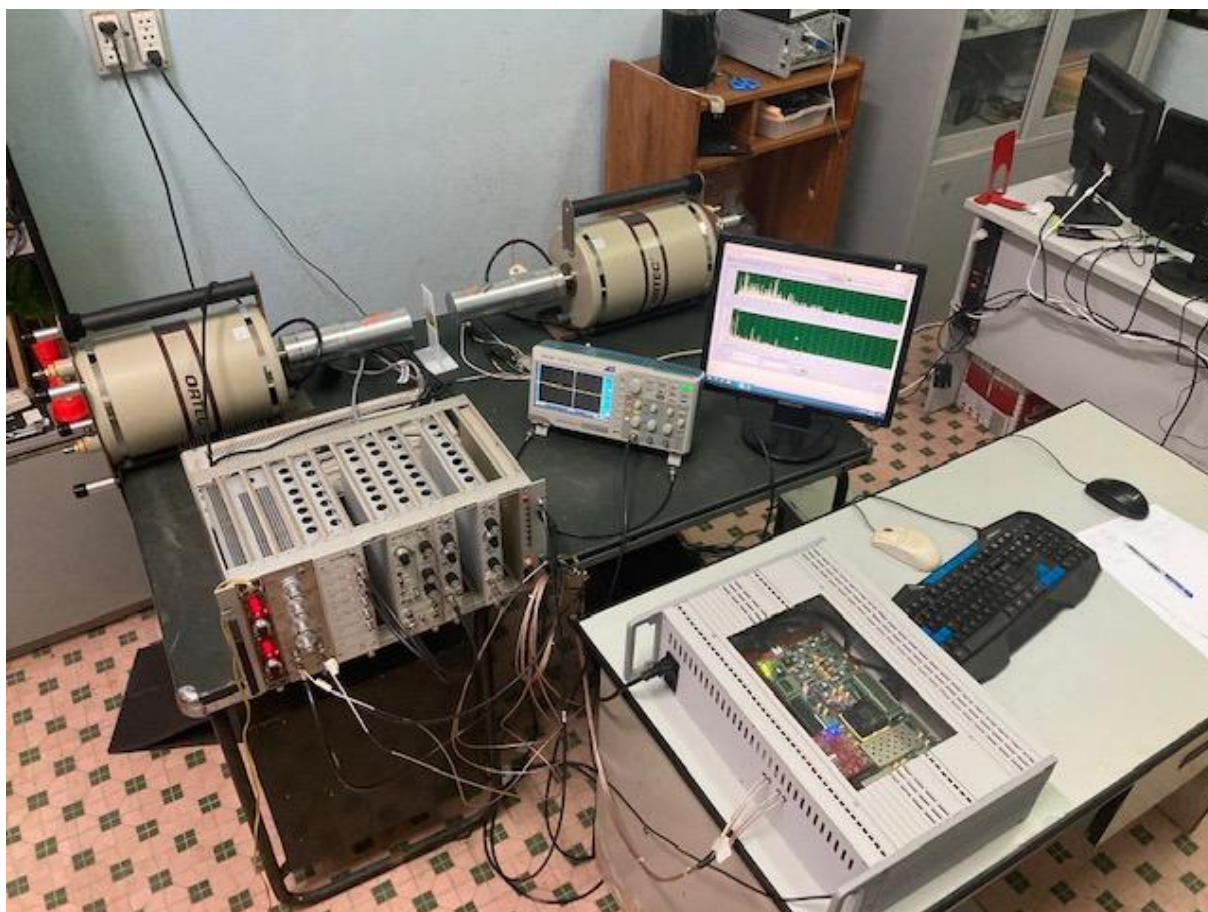
Digital gamma-gamma coincident spectrometer system, 4 channels 16K input (The product of State-level Project KC05.08/16-20 implemented by DNRI)
