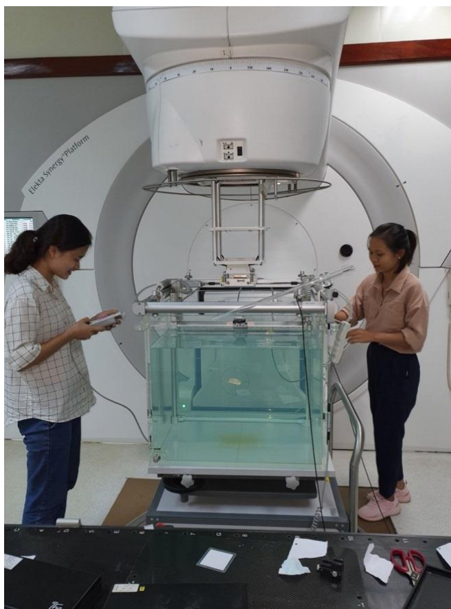
Radiation Safety Calibration of an Elekta Medical LINAC (Image credit: Center for Radiation Protection, INST)
