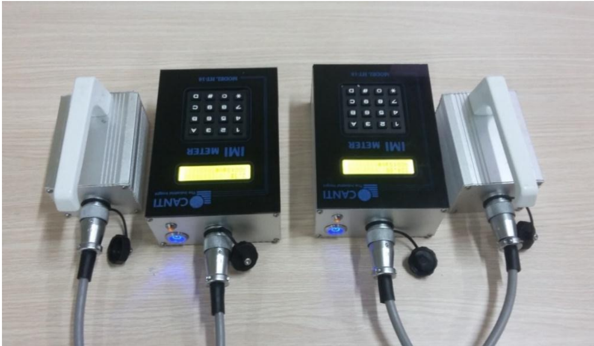
Conducting research and manufacturing IMI gauges for detecting carbon steel in stainless welds
