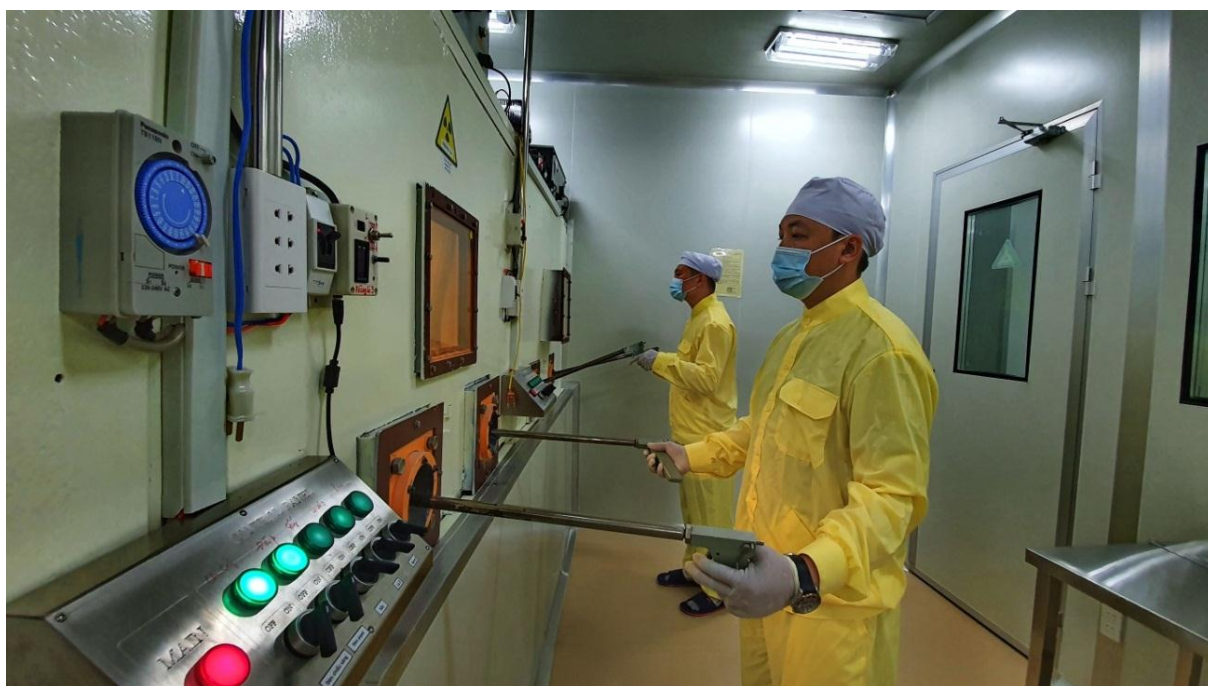
I-131 solution production line meets WHO-GMP standards at Dalat Nuclear Research Institute (DNRI)
