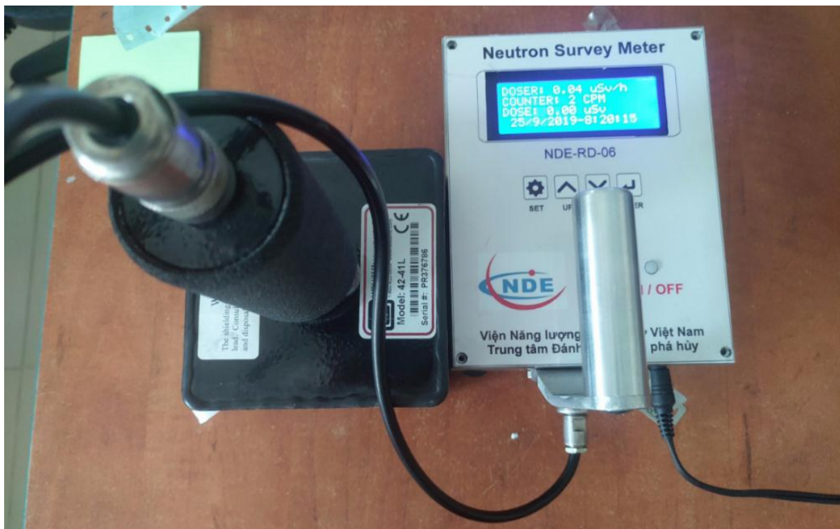
Neutron dosimeter device to control the dose of neutron radiation in industry in the Ministry-level project DTCB.02/17/TTNDE
