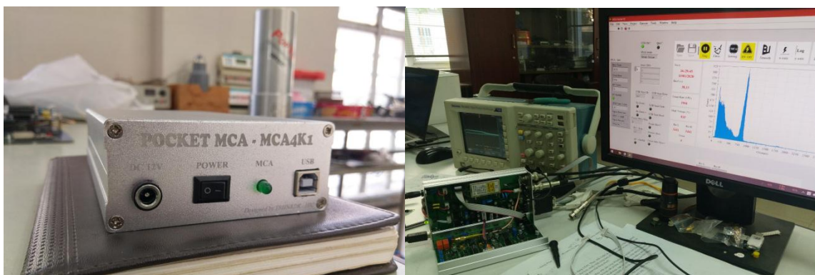
Manufacturing and testing of the POCKET MCA multichannel analyzer under a project in cooperation with the Institute of Nuclear Science and Technology
